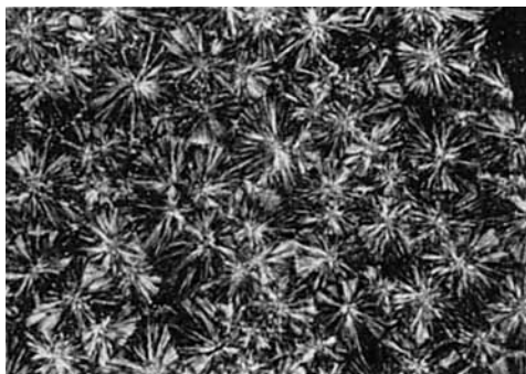
Fig. 1. Polypropylene film of fraction crystallized at 135°C. after aging in air for 5 days at 135°C.; as viewed through crossed nicols, 48X.
